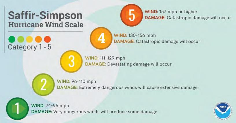
\* The Saffir/Simpson Hurricane Scale (shown above) can be used to estimate the potential property damage and flooding expected along the coast during a hurricane.
