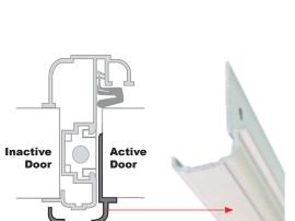
Add an Astragal Security Strip to any outswing double door combination for added security, a clean finished appearance, and eliminate the reveal between the doors.
