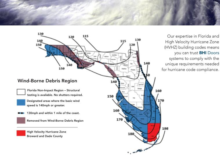
Impact units have structural ratings and may be used in the HVHZ and/or WBD impact zones without shutters required.
